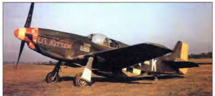
A P-51 B Li'l Kitten of the 357th FG with paint sand blasted on bottom surfaces because of forceful winds of the propeller.
