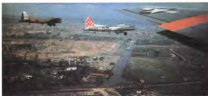
B-17's of the 385th BG have their gear down and bomb bay doors open to reduce speed at a food drop near Utrecht.
