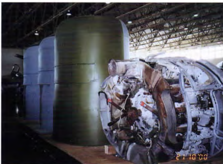
B-24 cowlings and engine from crash being restored at Hill Aerospace Museum
