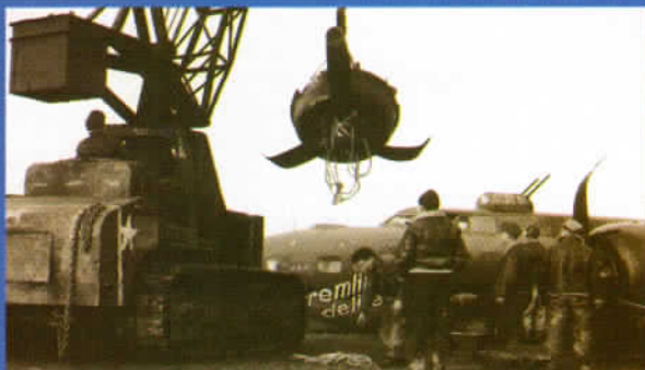
2nd S.A.D. Engine removal from belly landed "Gremlin Delite" 12-23-43, Ser. 42-3522
