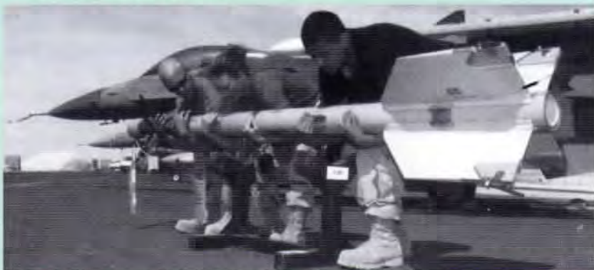
Weapons Specialists of the 379th Expeditionary Aircraft Maintenance Squadron hoist on AIM-9 Sidewinder missile before mounting it to an F-16 Fighting Falcon aircraft.
