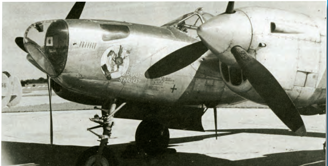
P-38 Lightning with Droop Snoot modification, carried a Norden bomb sight and bombardier in the nose. As lead plane a formation of P-38's would accurately drop 4,000 pounds of bombs on long range missions and then provide their own fighter coverage on their return home from the target. The Droop Snoot finished the war as a Photo Recon Group aircraft. —Editor
