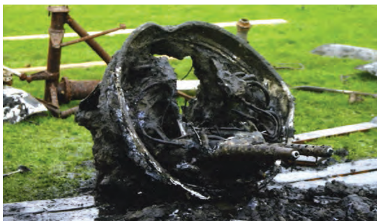
One of the remote-controlled gun barbettes with the twin .50s still in place.
