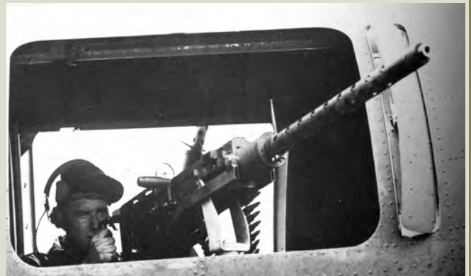
Note ring and post sight and charging handle on right side of breech mechanism on the right waist gun, manned by S/Sgt Louis Skinner of the 306th BG.
