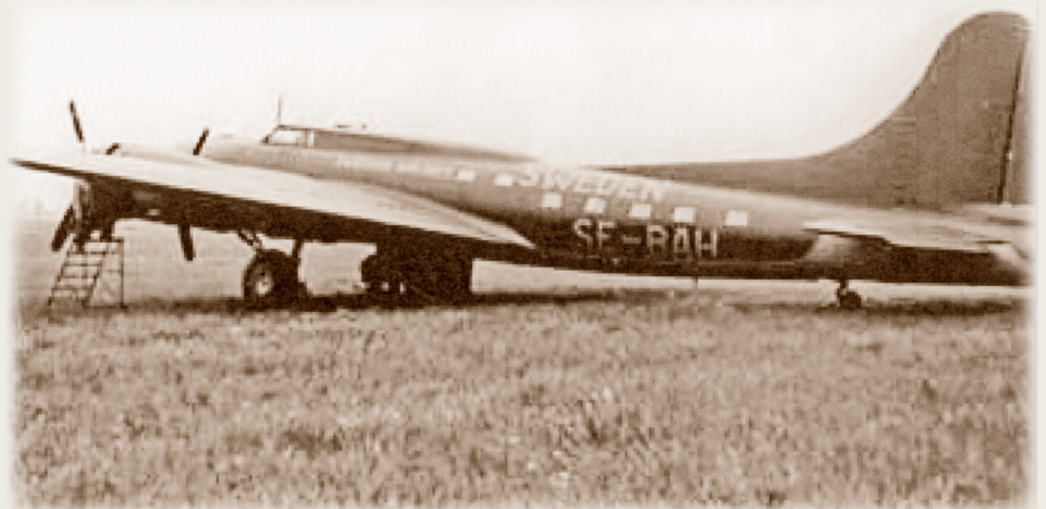
This Douglas-built B-17F was the first of seven former U.S. Army Air Force Flying Fortresses to be converted into a "Felix" airliner by Swedish aircraft and auto manufacturer Saab during World War II.
