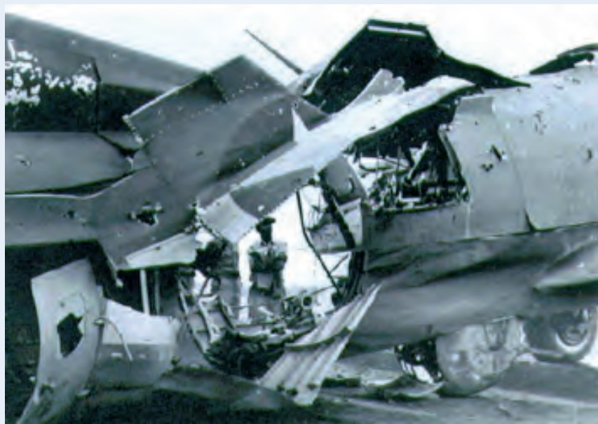
B17 G "Sweet Pea" returned to Amendola air base in Foggia, Italy and immediately upon landing, came to a stop and collapsed as you see it here. This was following a direct hit from an 88mm flak shell which exploded in the aircraft's middle section.
